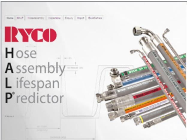
Hose Assembly Lifespan Predictor, an online program that predicts the lifespan of hose assemblies for given conditions and environments.
